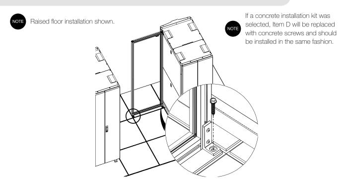
Using a drill, 1/2" deep socket, and 1/2" x 2" self tapping screws (Item D), fasten the frame down in the (2) locations where pilot holes were drilled.
