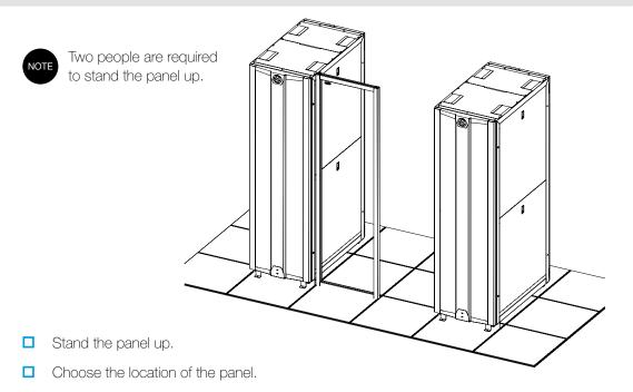
☐ The location of the panel will vary based upon the overall design of the containment solution.
