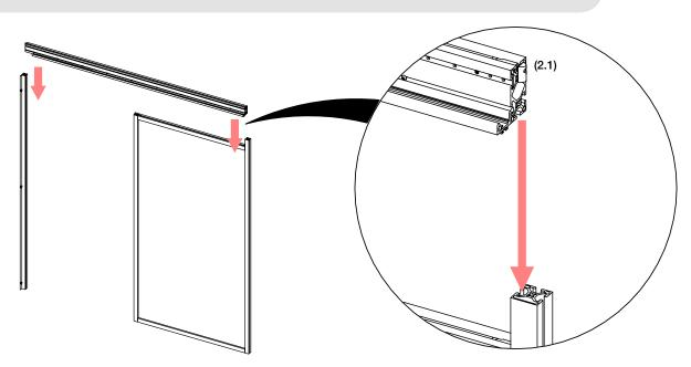
(2.1) Slide the t-nut on the Header in the slot of the frame on both sides of the Header.
