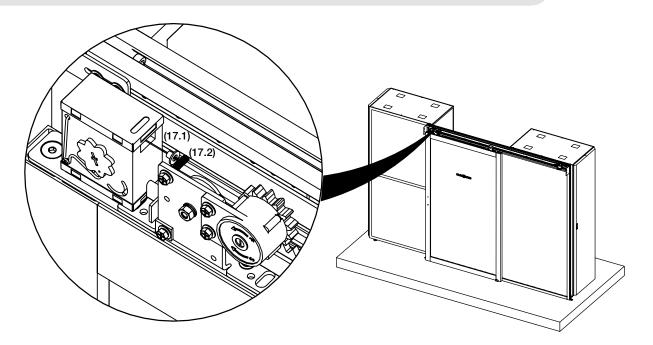
(17.1) Pull out the chord on the Pull Spring.
