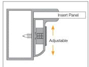
ACT is an adjustable, twopiece extrusion capable of accommodating panel insert thicknesses from 1/8" to 3/8"
