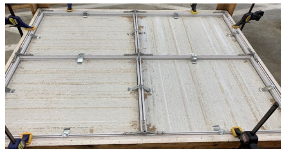
FIGURE 7 Ultima AirAssure gasketed tile with DynaMax grid in leakage test fixture. The combination reduces leakage at the tile perimeter and eliminates leakage around drop rods, providing the best containment possible to-date.
